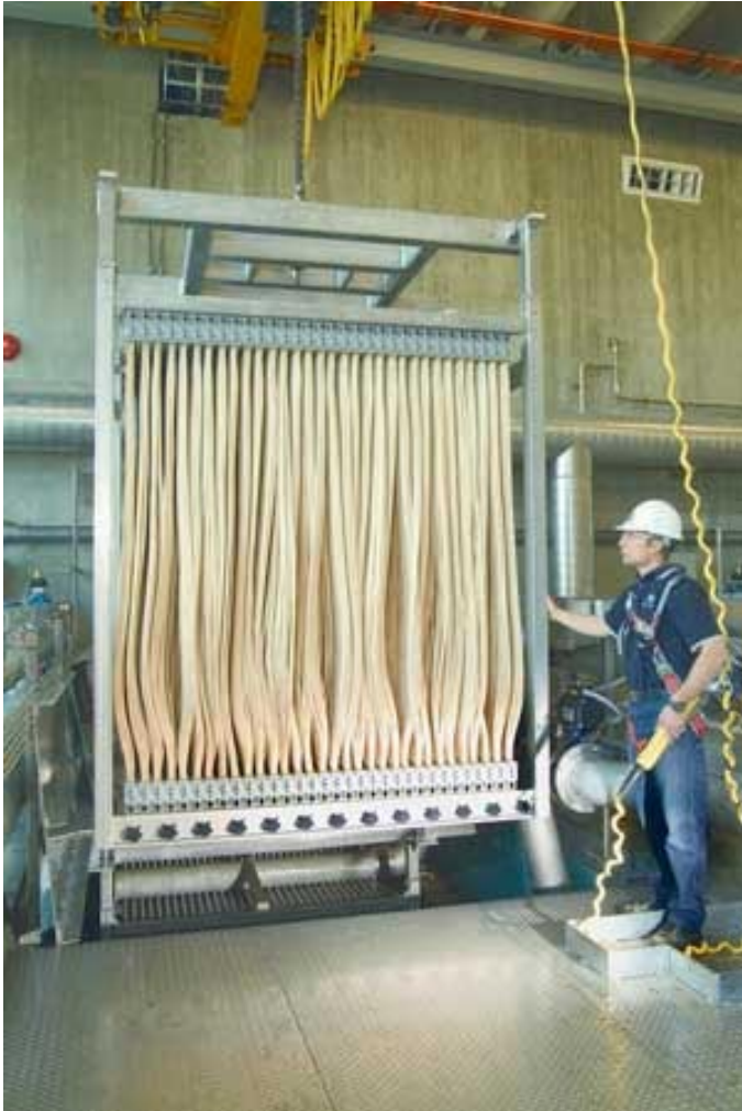
Membranes for recovering water from sewage in King County, Washington
