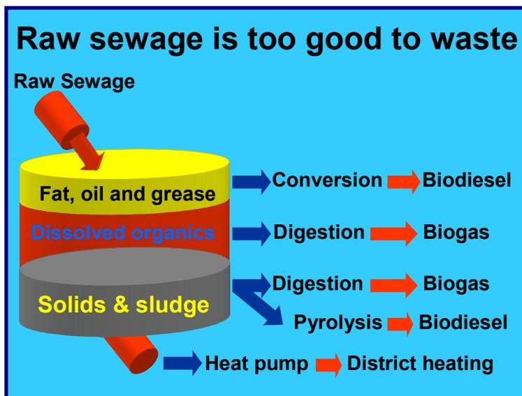
In anaerobic treatment plants on the other hand, methanogenic bacteria digest organic materials and produce raw biogas - a mixture of roughly 1/3 CO<sub>2</sub> and 2/3 methane. When the raw gas is stripped of CO<sub>2</sub> and trace sulphur compounds (using treated wastewater) the resulting natural gas can be distributed for use in homes or cars.
